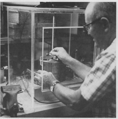
KRYPTON 85 content of each cell can be calculated through use of a calorimeter. Alex Thom (1626-3) places a dead cell in one of copper cylinder's two wells. A hot cell will be inserted in other well.
